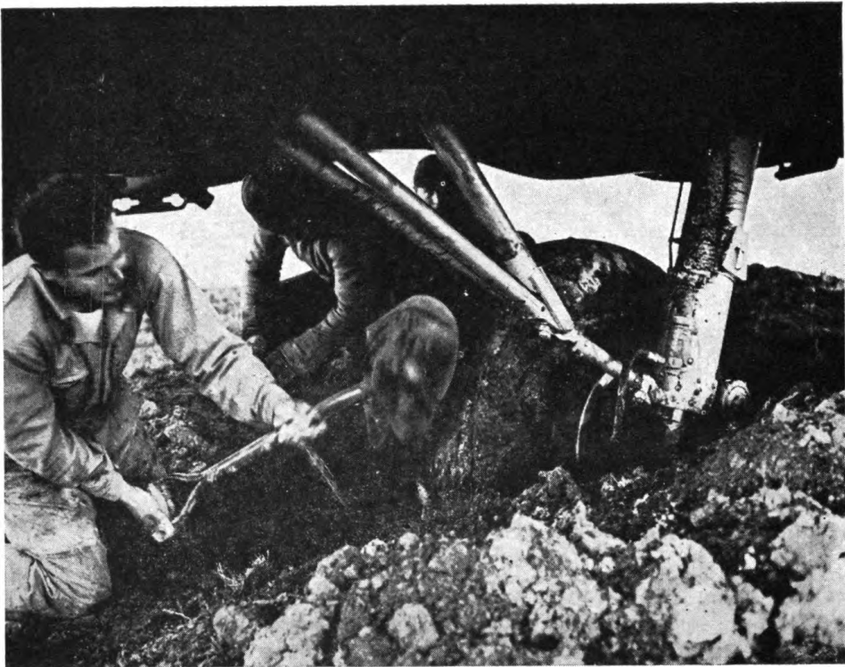
Figure 186. Failure of natural surface. Plane has bogged down where it left surface runway.
